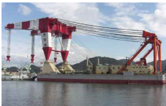
(a) 低頭式起重機：羽田D滑走路[6]
