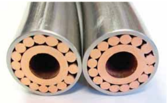
Model CORC ® -CICC made with copper strands [AC1]
