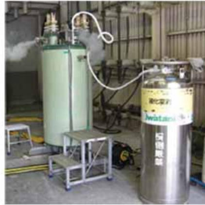
Fig. 1. Photograph of a 1 \phi -6.9 kV/2.3 kV-400 kVA transformer [5], [6].
